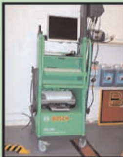
MAHA Equipment and Bosch Smoke Tester as used by SGS
