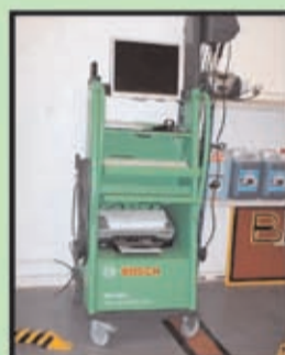
MAHA Equipment and Bosch Smoke Tester as used by SGS
